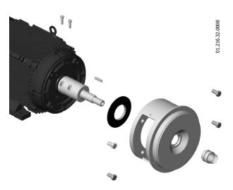
10. Loosen the allen screws (51A) securing the shaft (05) to the motor (93). If you cannot take out the shaft (05), introduce a screw in the first hole to help extract it.
